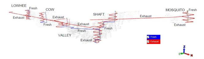
Figure 16-39: General view of the Cariboo ventilation network (N-E view)
