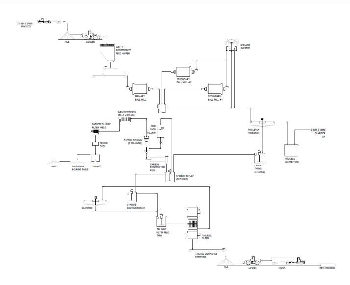
Figure 17-2: The QR Mill simplified process flow diagram
