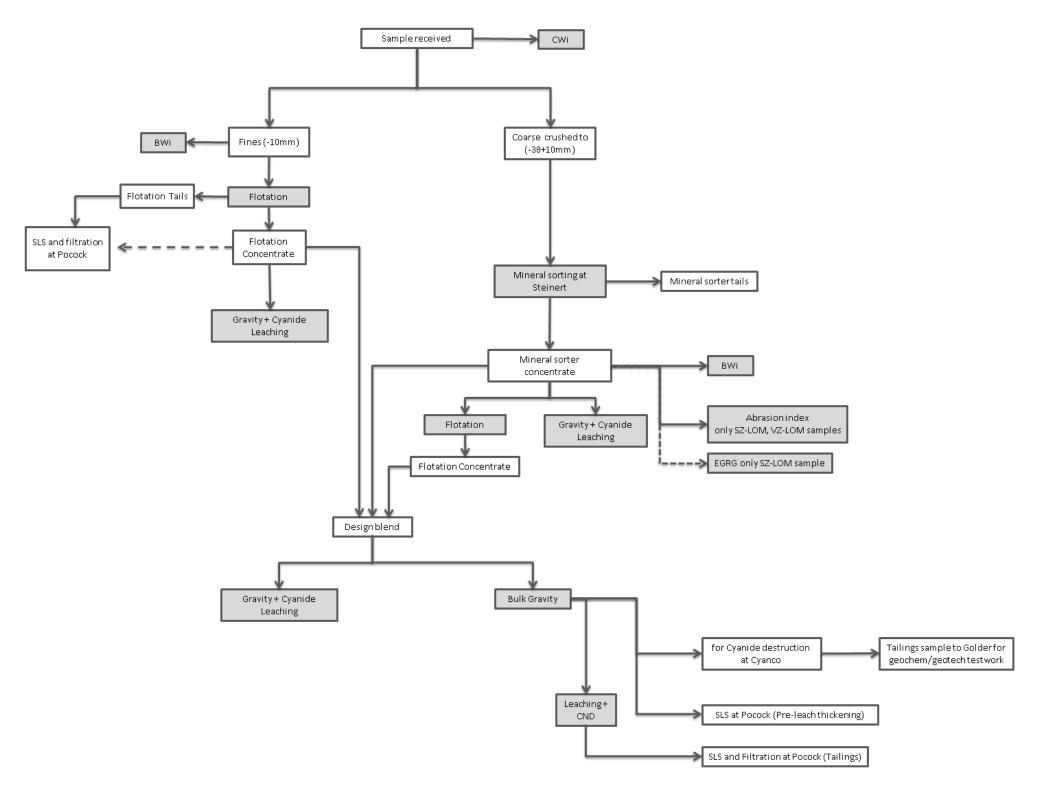
Figure 13-3: Testwork program map and samples produced for extended testwork (Source: Morgan et al, 2019)
