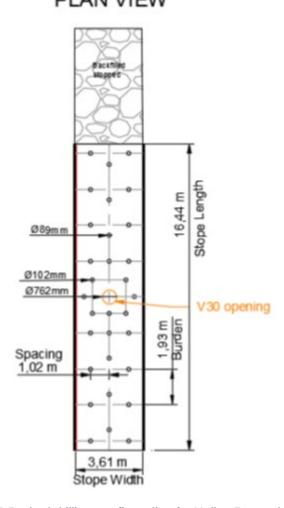
Figure 16-17: Typical drilling configuration for Valley Zone, plan view
