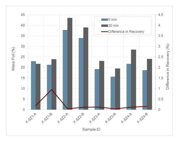
Figure 13-8: Impact of flotation time on mass pull and gold recovery (Hansuld and Gajo, 2019)
