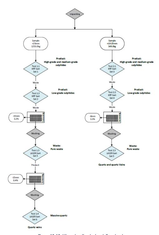
Figure 13-12: Mineral sorting testwork flowsheet (Source: Shibistova, 2021)
