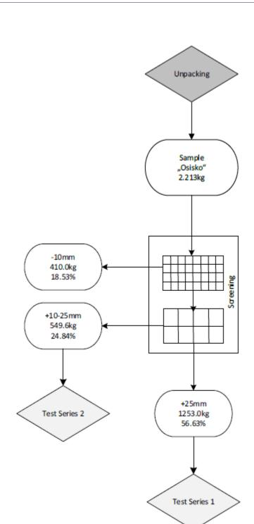
Figure 13-11: Sample preparation flow diagram (Source: Shibistova, 2021)
