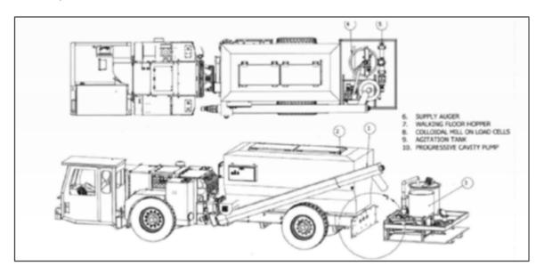
Figure 16-34: Convertible shotcrete mobile unit
