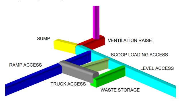
Figure 16-16: Isometric view of typical truck loading area
