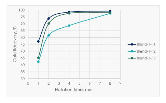
Figure 13-14: Flotation time versus gold recovery – Blend 1
