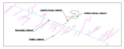
Figure 16-33: Isometric view of typical network distribution – Level 1240 (Cow Zone)
