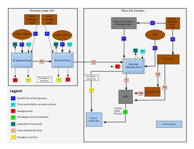
Figure 20-1: Flow diagram at Mine Site during operations
