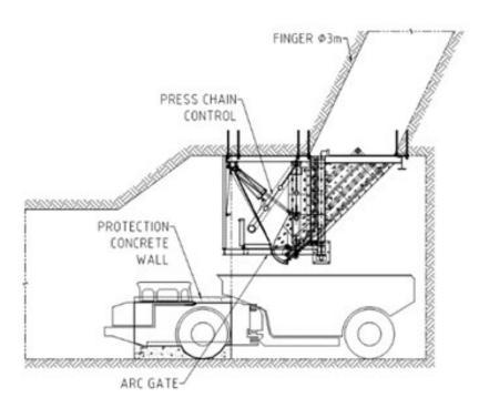
Figure 16-31: Waste truck chute
