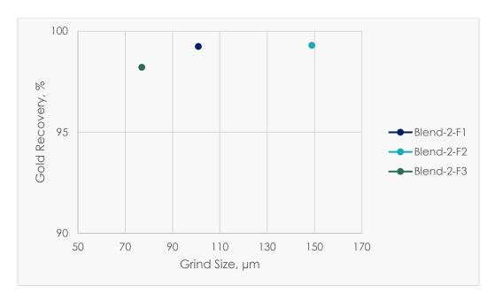
Figure 13-18: Grind size versus gold recovery - Blend 2
