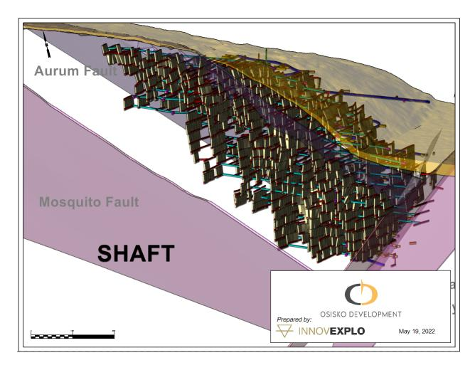
Figure 16-20: Perspective view of Shaft Zone showing traversing fault structures, looking north
