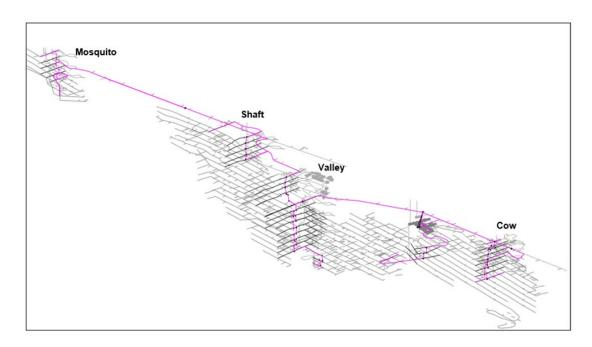
Figure 16-32: Longitudinal View of Paste Network for Cariboo Project
