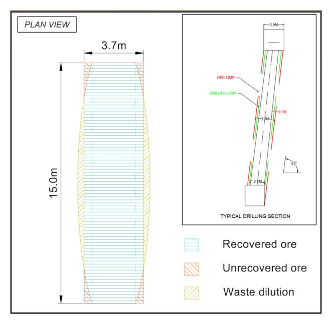
Figure 16-29: Internal dilutions strategy for stopes wider than the minimum mining width
