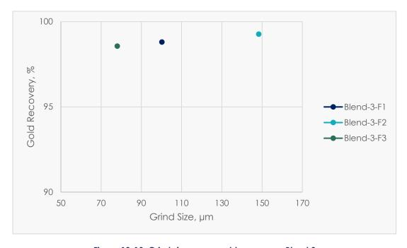
Figure 13-19: Grind size versus gold recovery – Blend 3
