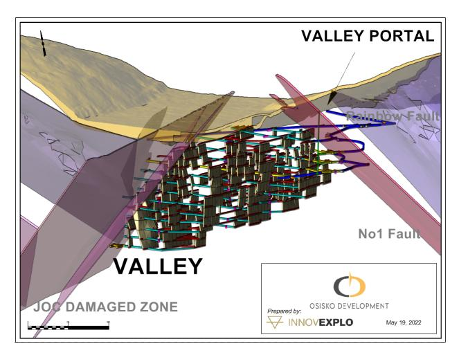
Figure 16-22: View of Valley Zone showing traversing fault structures, looking north
