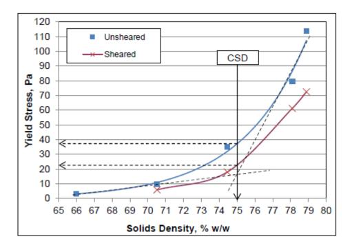
Figure 13-27: Yield stress versus solids density – Flotation concentrate underflow (Source: Liu and Ashbury, 2022)
