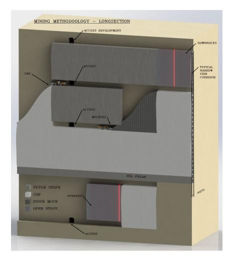
Figure 16-12: Longitudinal longhole retreat – Long section
