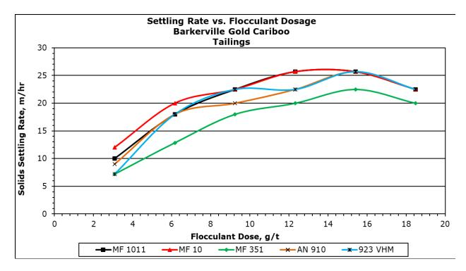
Figure 13-26: Settling rate vs Flocculant dosage (Source: De Paula, 2022)
