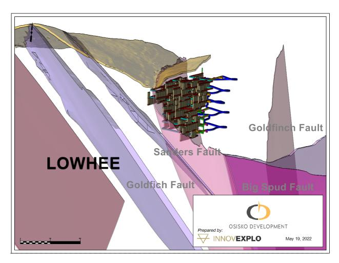
Figure 16-26: Perspective view of Lowhee Zone looking northeast showing fault structures
