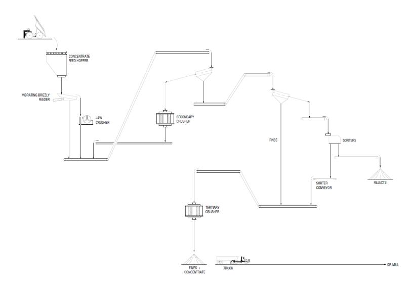
Figure 17-1: Bonanza Ledge Site simplified process flow diagram
