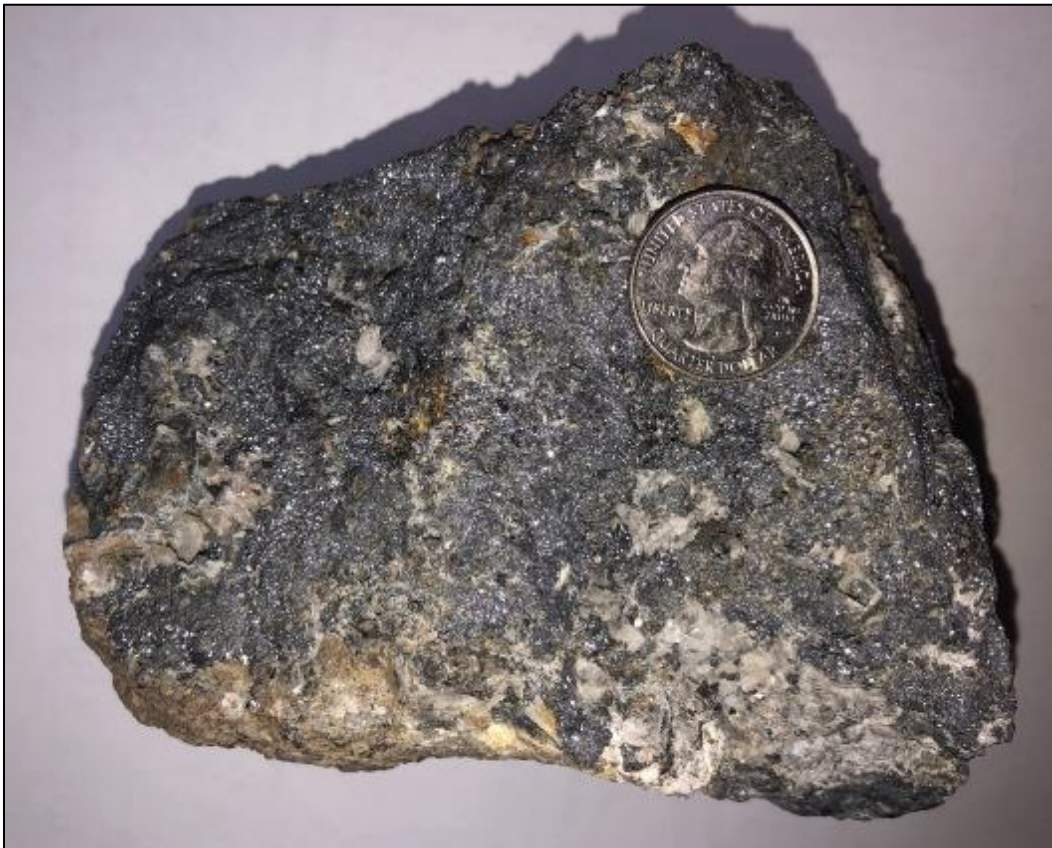
Figure 8.2 CRD-Style Base-Metal Mineralization, Massive Galena Typical of the Historic Burgin, Tintic Standard and North Lily Mines
