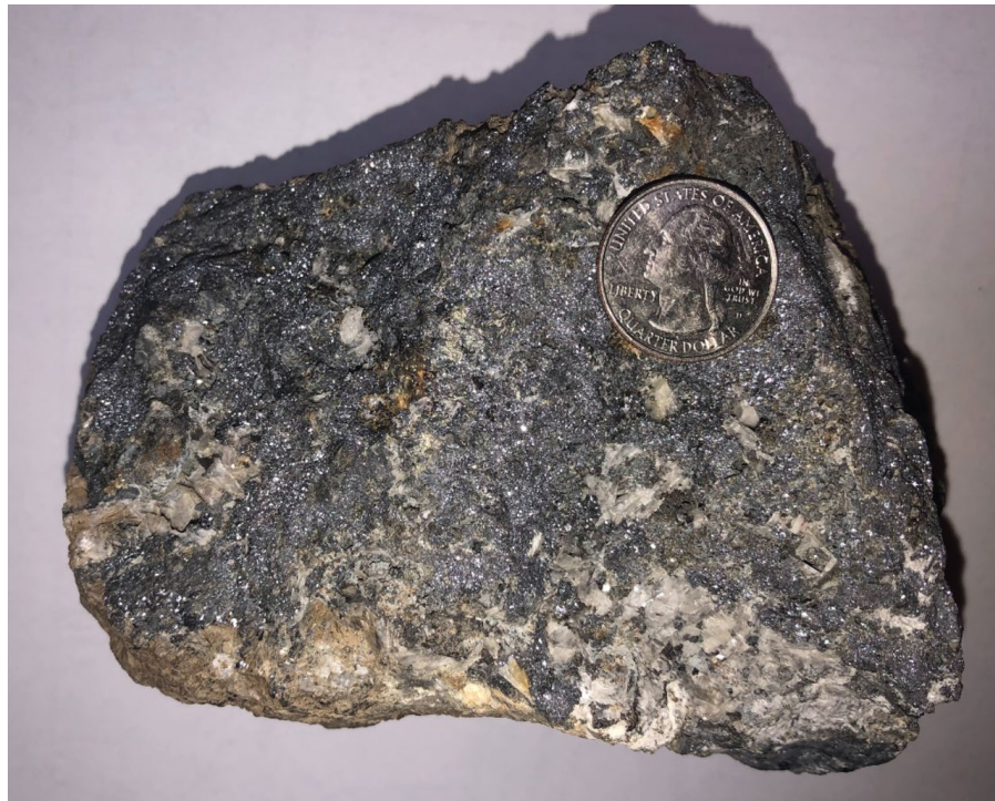
Figure 8-2: Photo of CRD-style base-metal mineralization, massive galena (Pb-ore) typical of the historic Burgin and Tintic Standard mines
