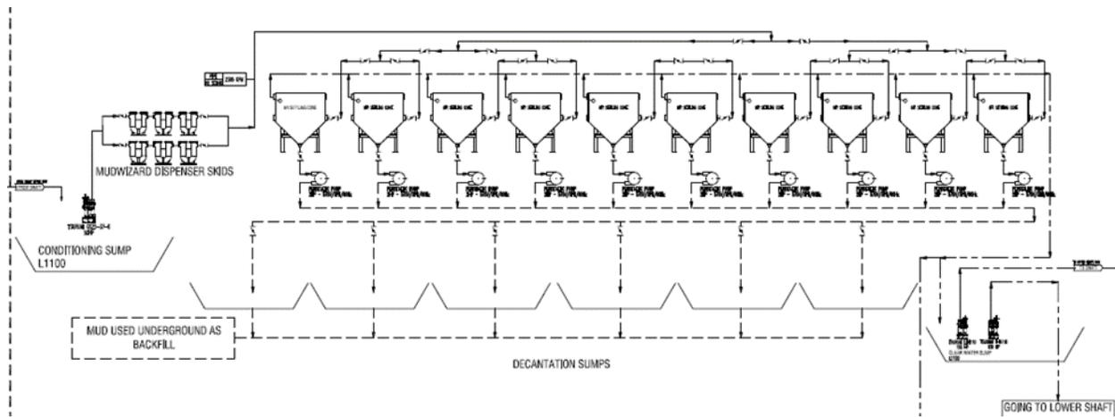
Figure 16-42: Clarification System Schematic (Partial)
