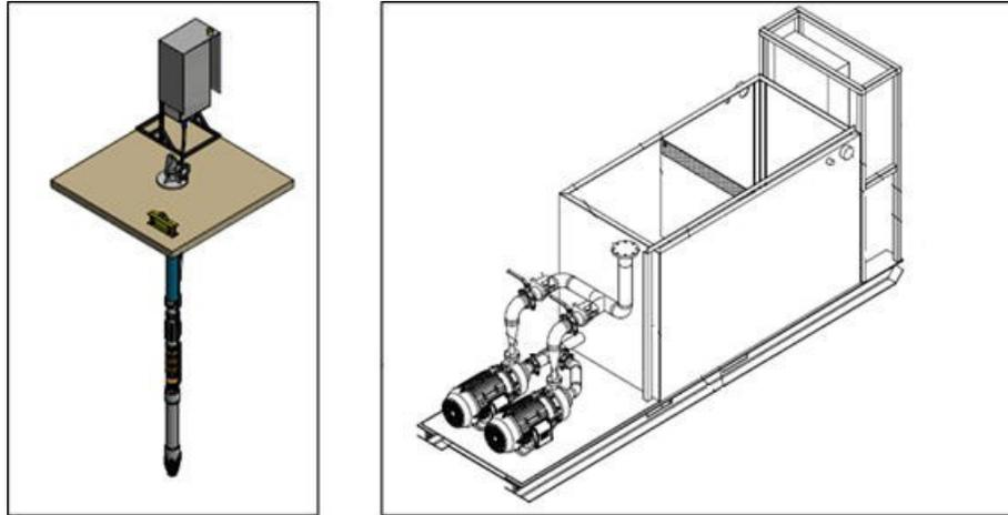
**Figure 16-41: TechnoSub proposed solution for flooded workings – Deepwell pump (left) and U/G pump station (right)**
