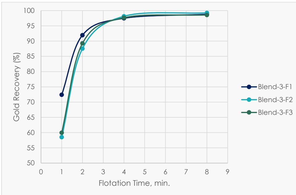
Figure 13-16: Flotation time versus gold recovery – Blend 3
