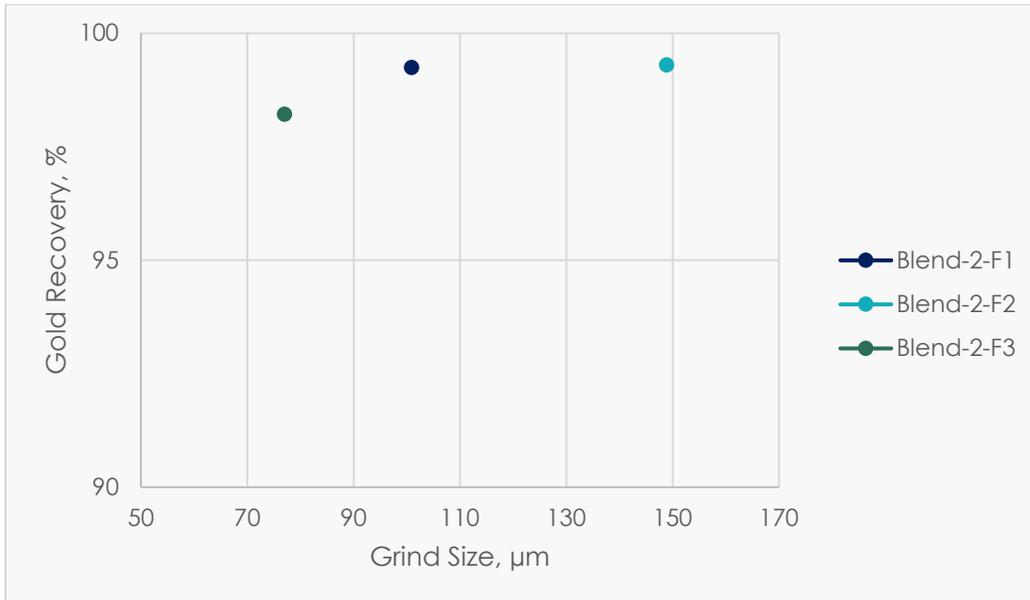
Figure 13-18: Grind size versus gold recovery – Blend 2
