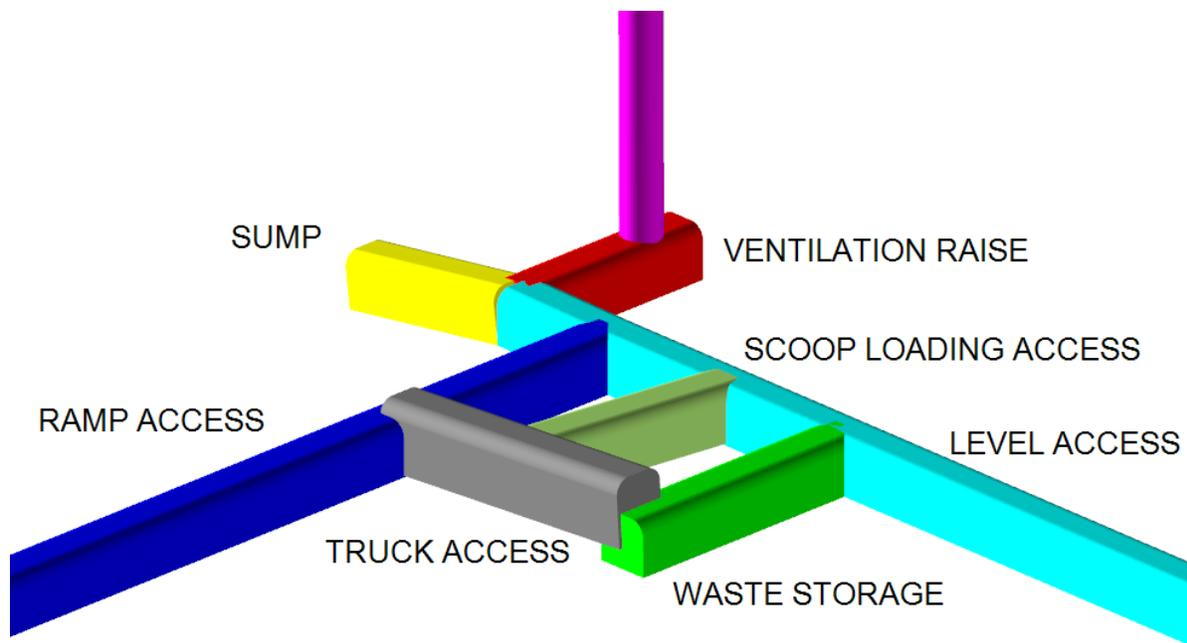
Figure 16-16: Isometric view of typical truck loading area
