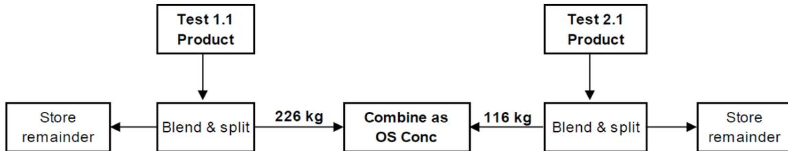
**Figure 13-13: Sample preparation – Mineral sorter concentrate**
