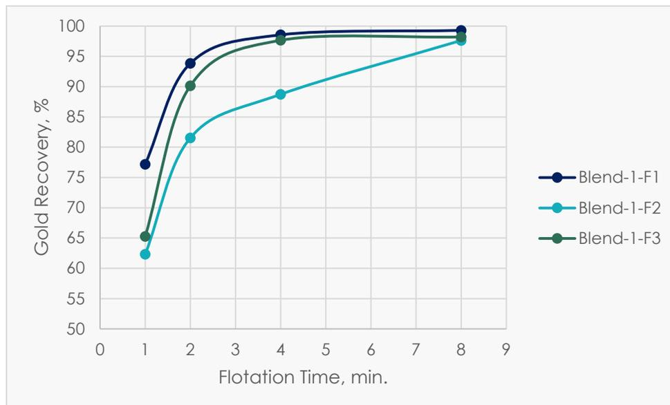
Figure 13-14: Flotation time versus gold recovery – Blend 1
