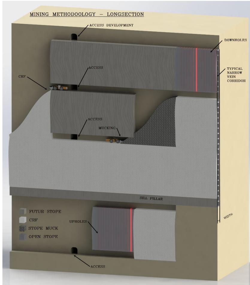
Figure 16-12: Longitudinal longhole retreat – Long section
