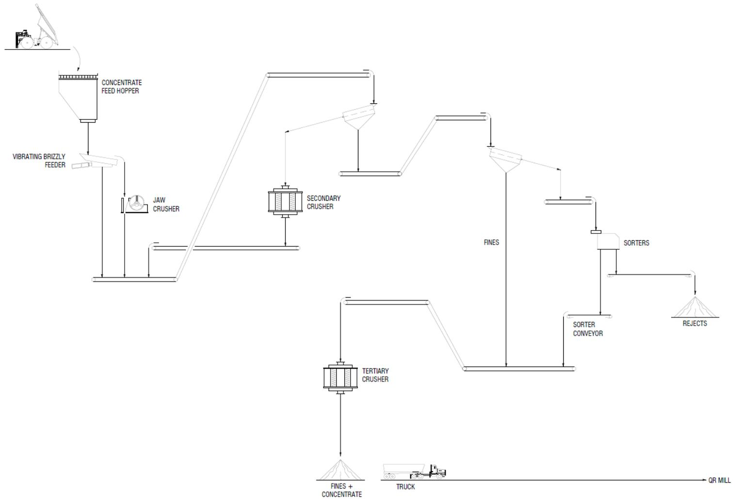
Figure 17-1: Bonanza Ledge Site simplified process flow diagram
