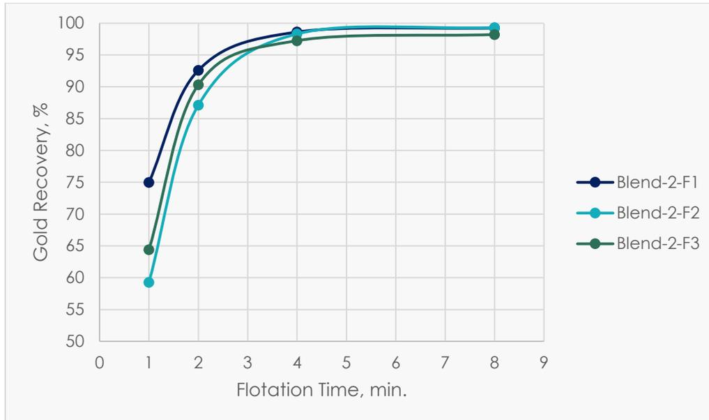
Figure 13-15: Flotation time versus gold recovery – Blend 2
