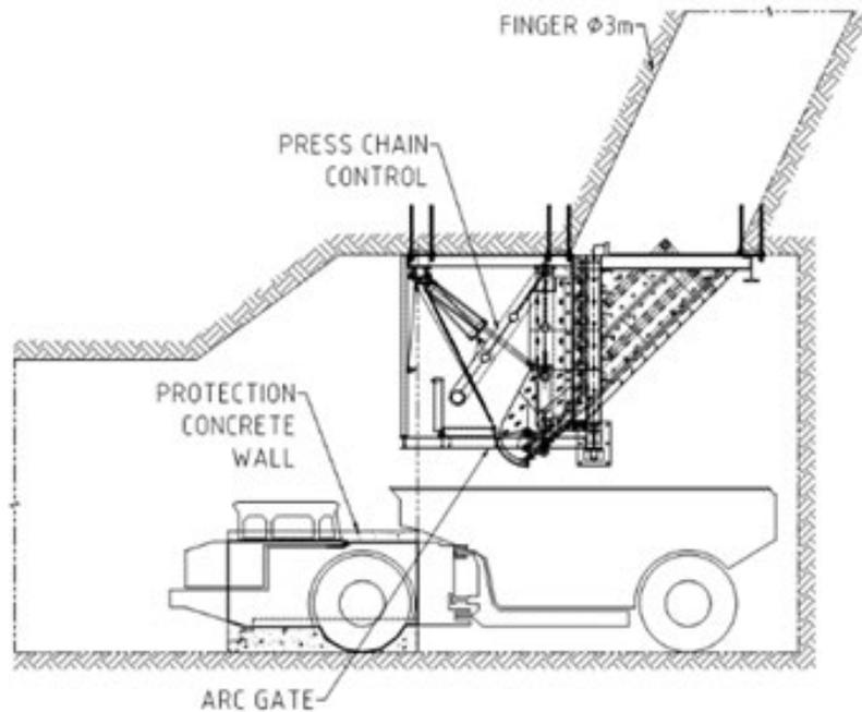
Figure 16-31: Waste truck chute
