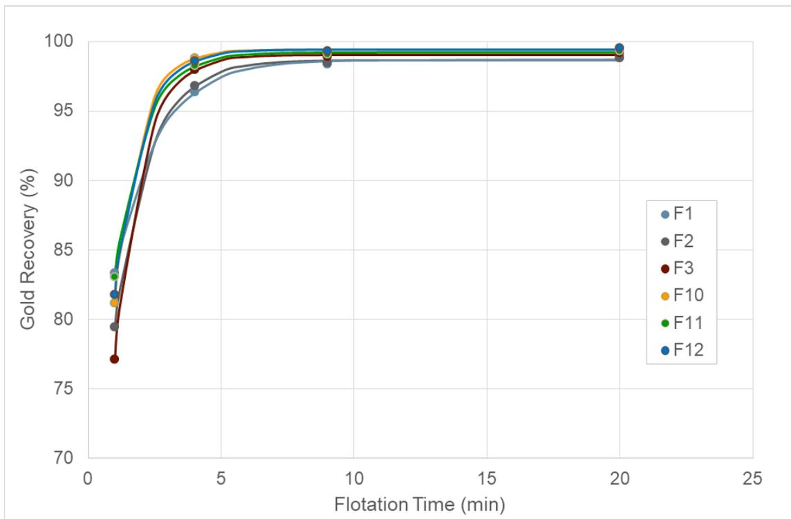
**Figure 13-7: Gold recovery flotation kinetics
