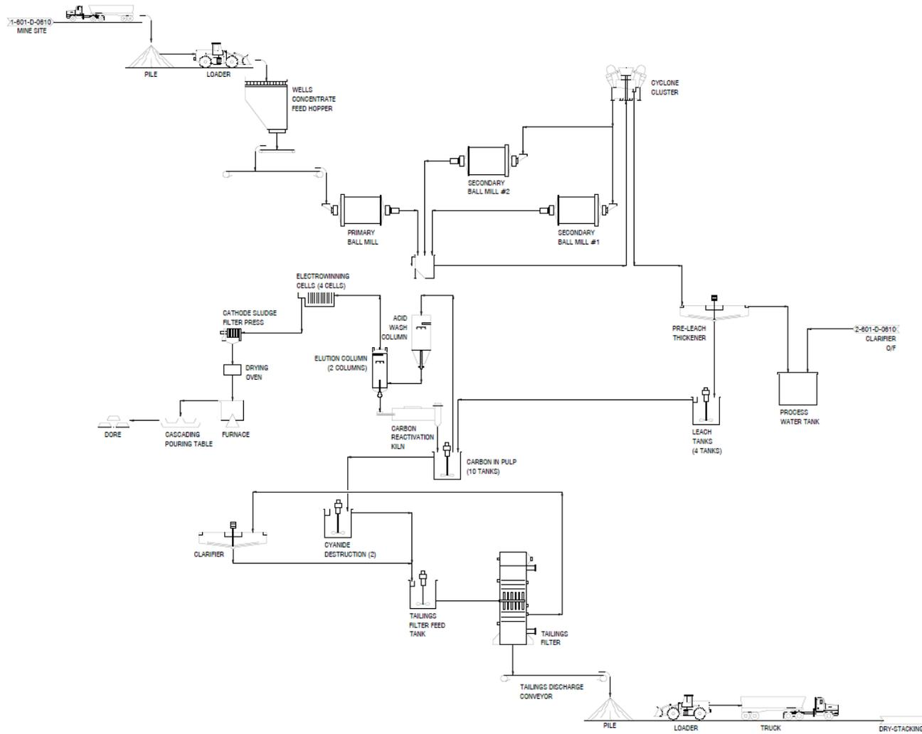
Figure 17-2: The QR Mill simplified process flow diagram
