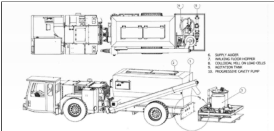
Figure 16-34: Convertible shotcrete mobile unit
