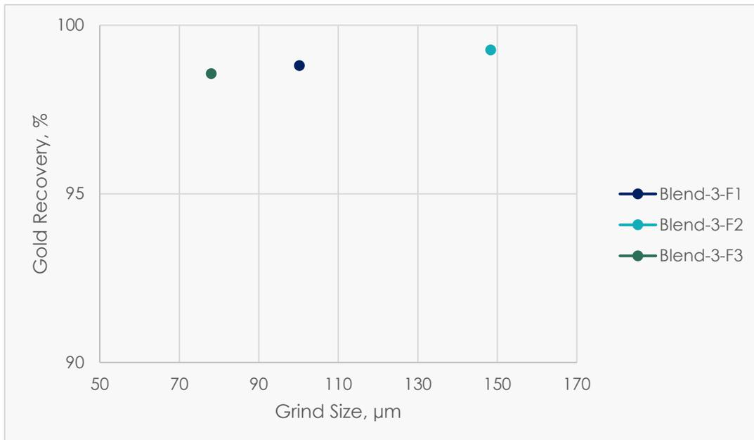
Figure 13-19: Grind size versus gold recovery – Blend 3
