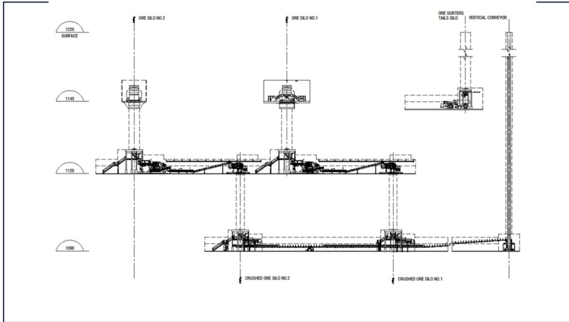
Figure 16-30: Elevation view of the U/G mineralized material and waste handling
