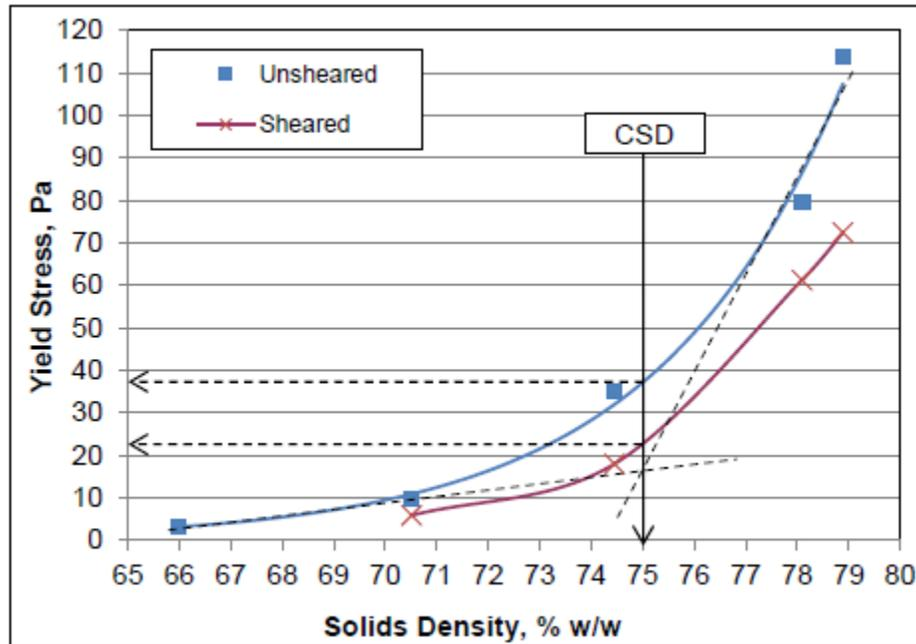
Figure 13-27: Yield stress versus solids density – Flotation concentrate underflow
