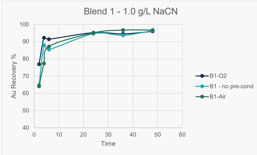
Figure 13-21: Leach kinetics for blend 1 at 1.0 g/L NaCN
