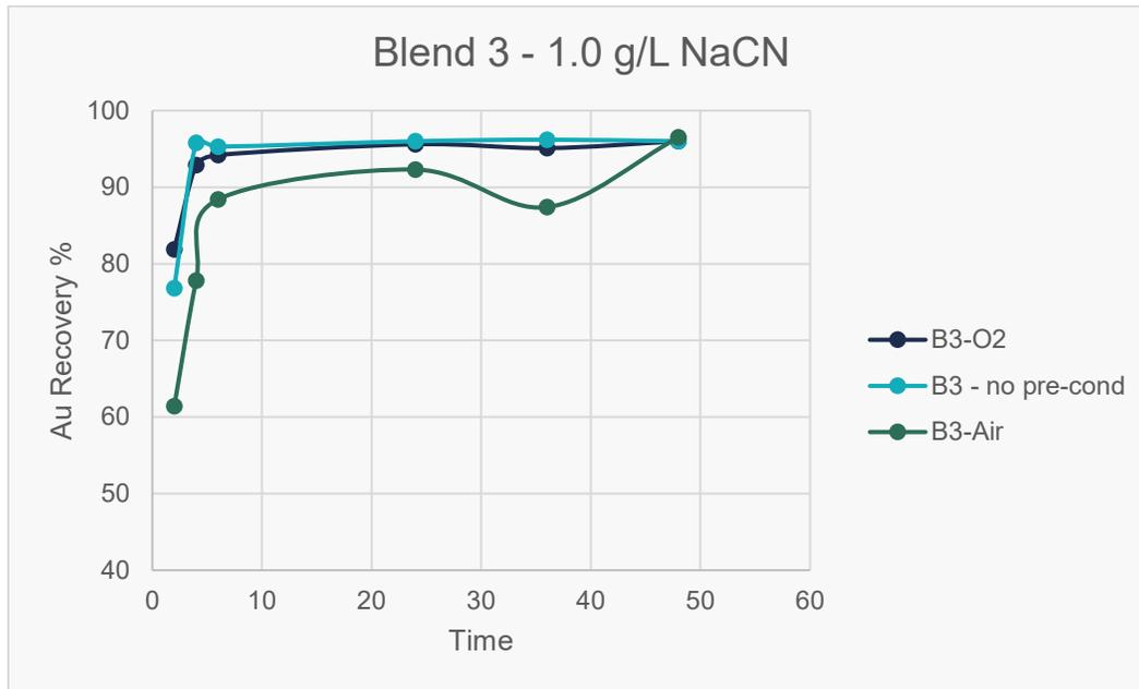
**Figure 13-23: Leach kinetics for blend 3 at 1.0 g/L NaCN**
