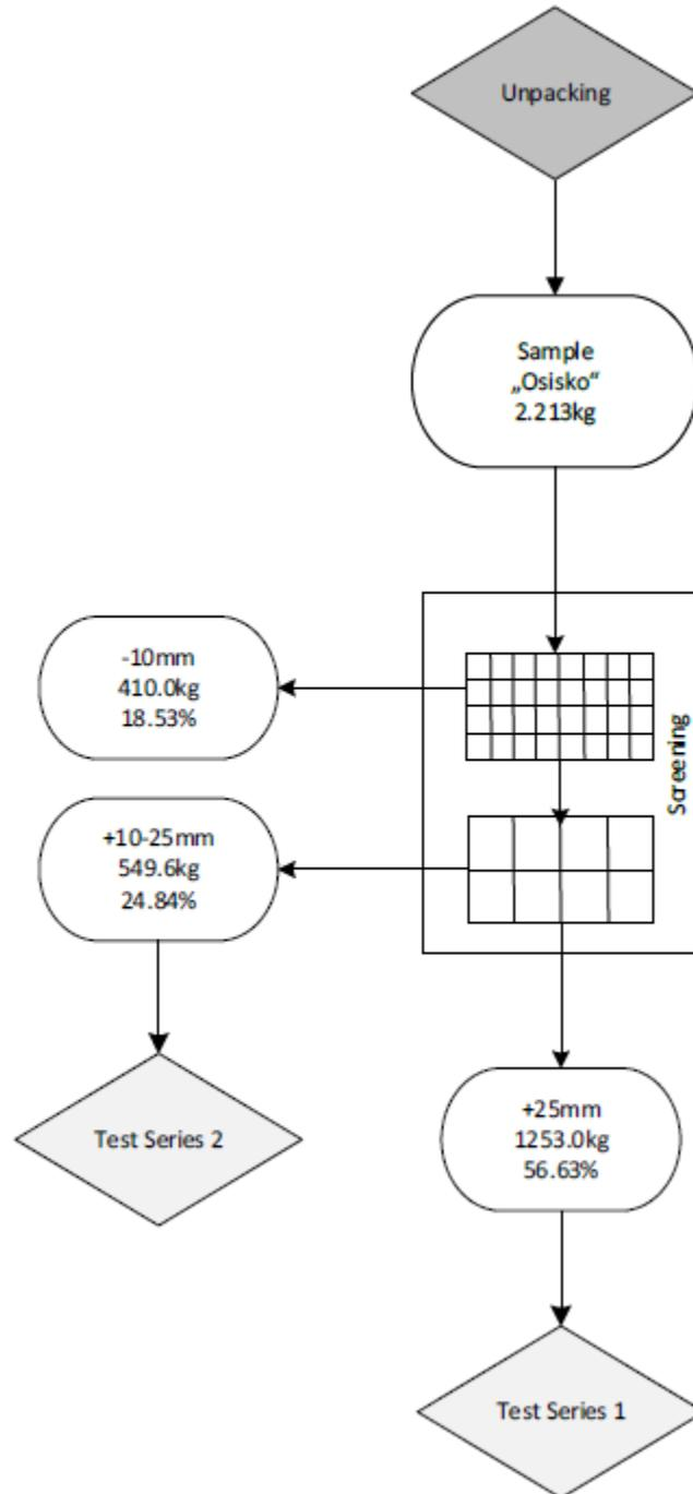
Figure 13-11: Sample preparation flow diagram
