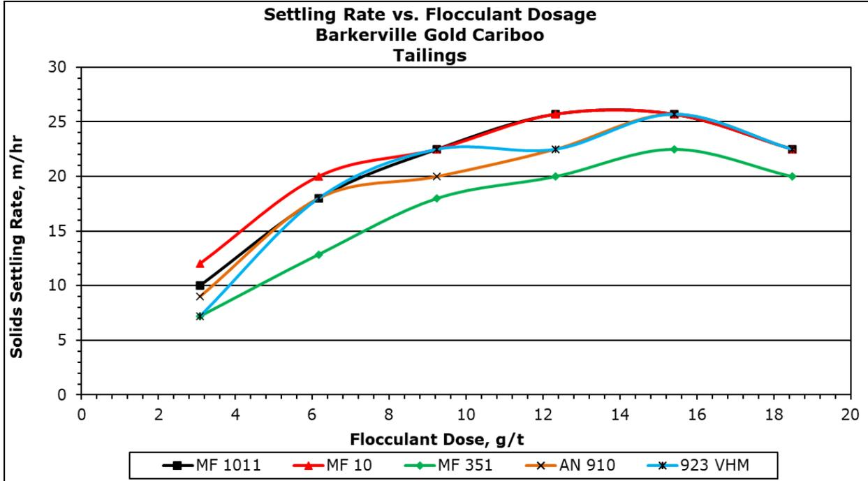
Figure 13-26: Settling rate vs Flocculant dosage
