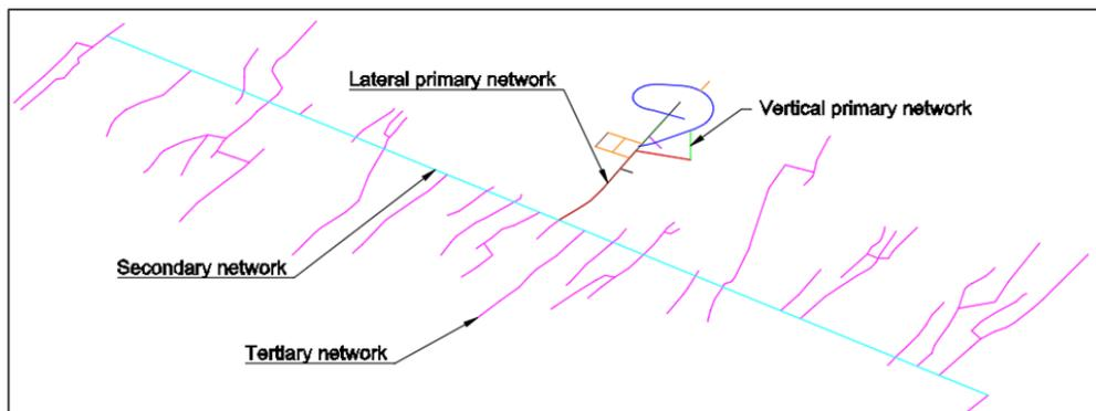
**Figure 16-33: Isometric view of typical network distribution – Level 1240 (Cow Zone)**
