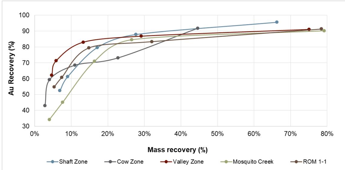
**Figure 13-6: Mineral sorting grade recovery curves**
