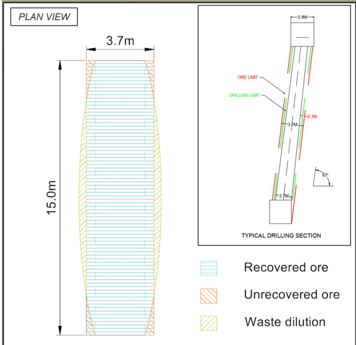
Figure 16-29: Internal dilutions strategy for stopes wider than the minimum mining width
