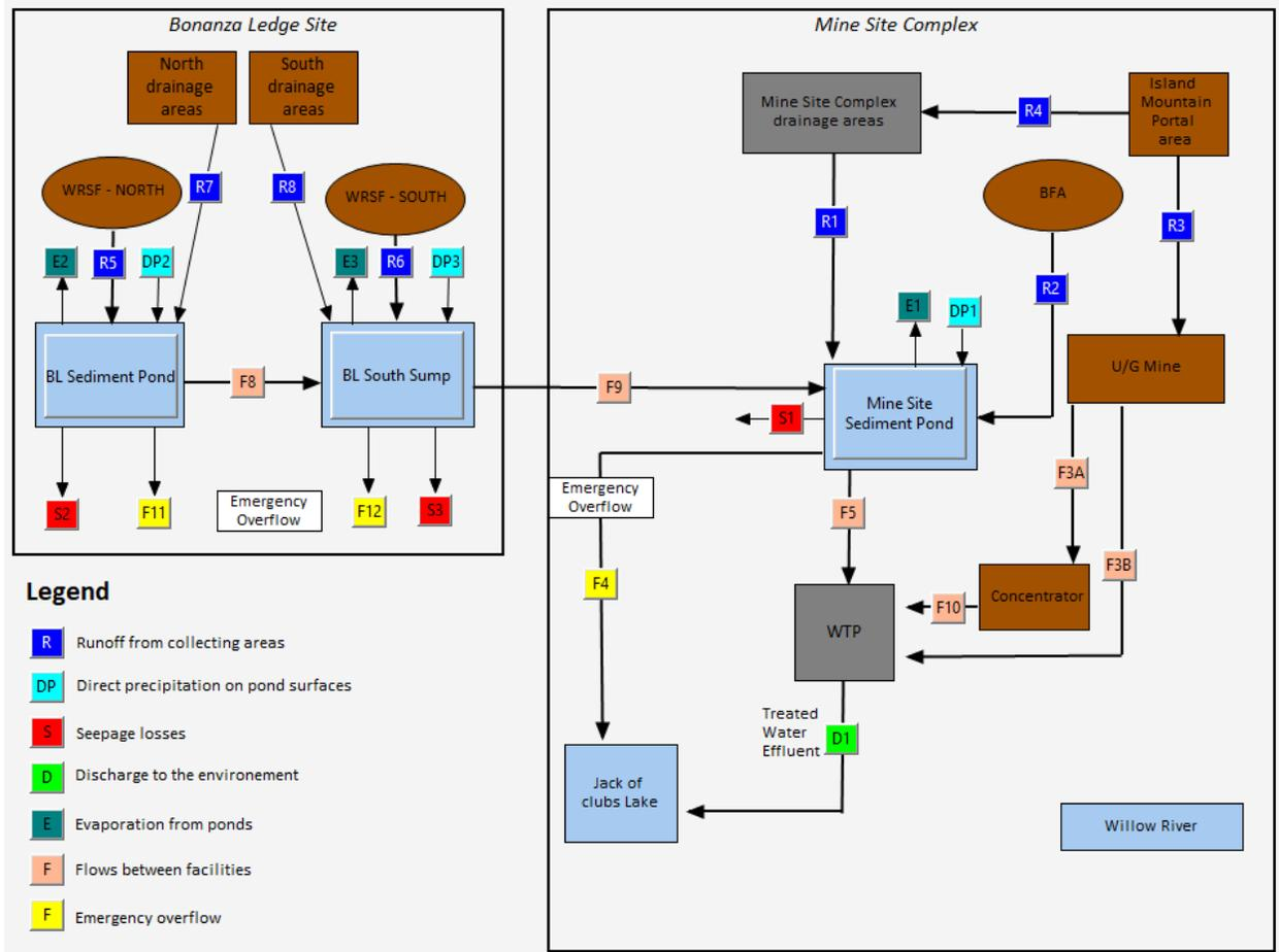
Figure 20-1: Flow diagram at Mine Site during operations
