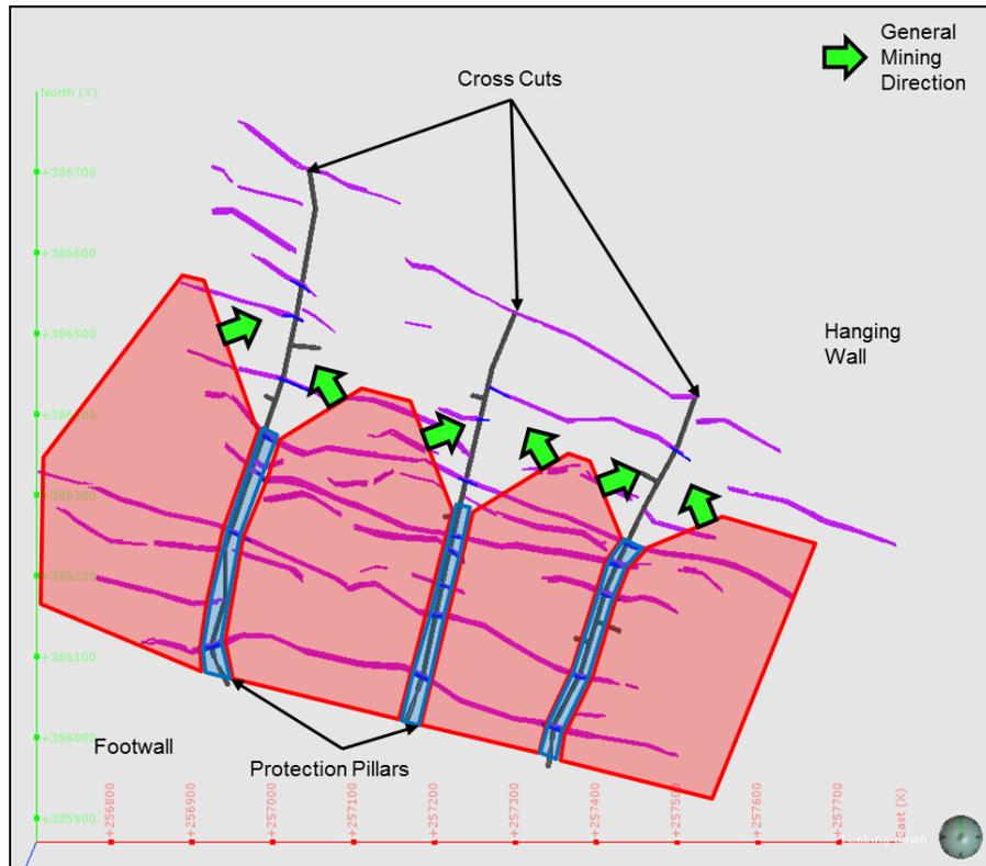
Figure 16-2: Schematic of the recommended general extraction sequence, with protection pillars being retained along the cross cuts
