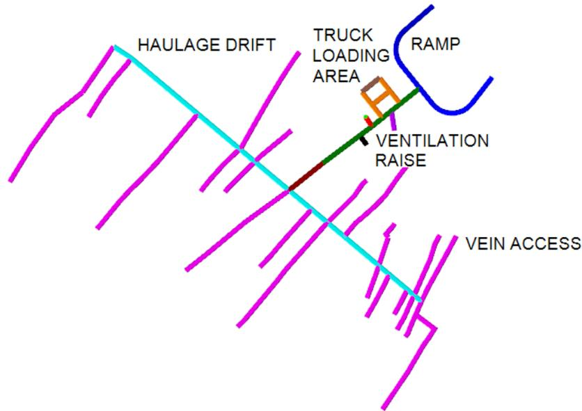
**Figure 16-15: Plan view of typical level layout**
