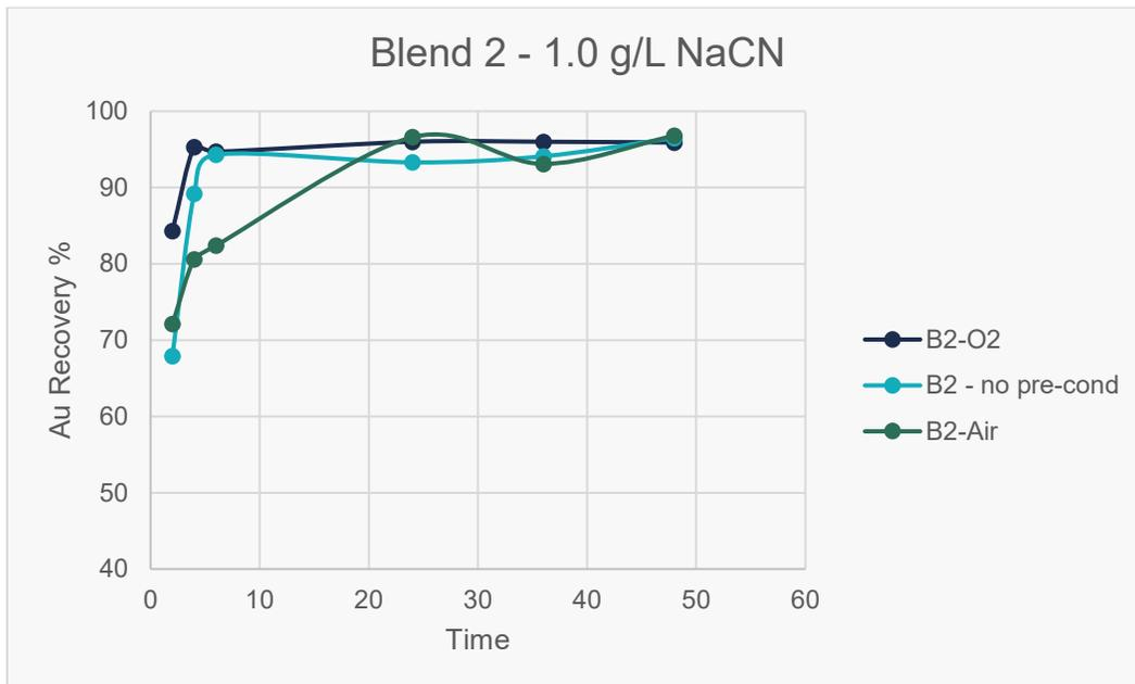
Figure 13-22: Leach kinetics for blend 2 at 1.0 g/L NaCN
