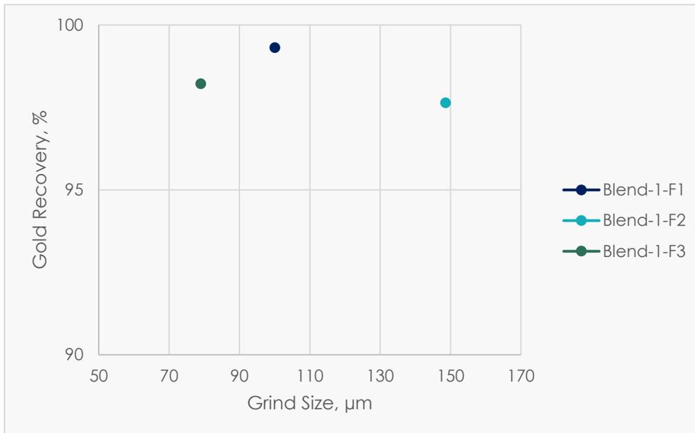
Figure 13-17: Grind size versus gold recovery – Blend 1
