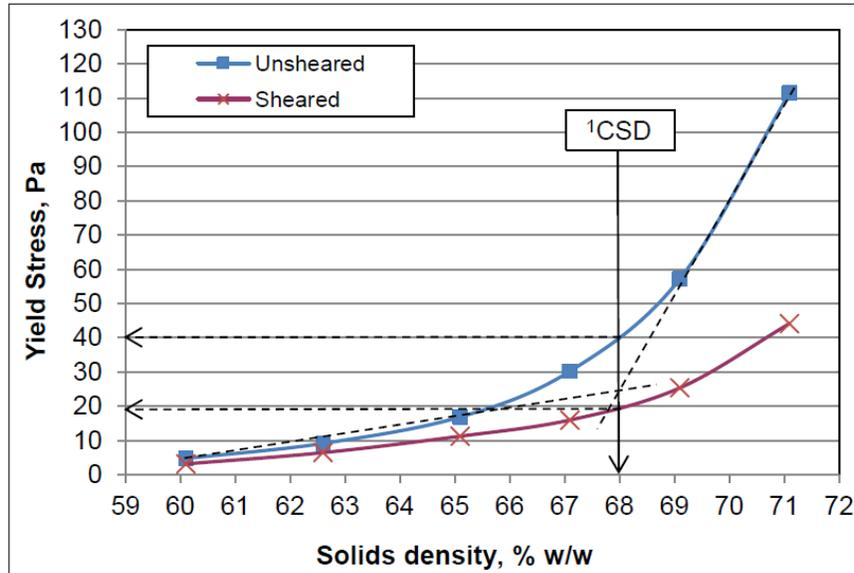
Figure 13-28: Yield stress versus solids density – CIP detox tailings underflow
