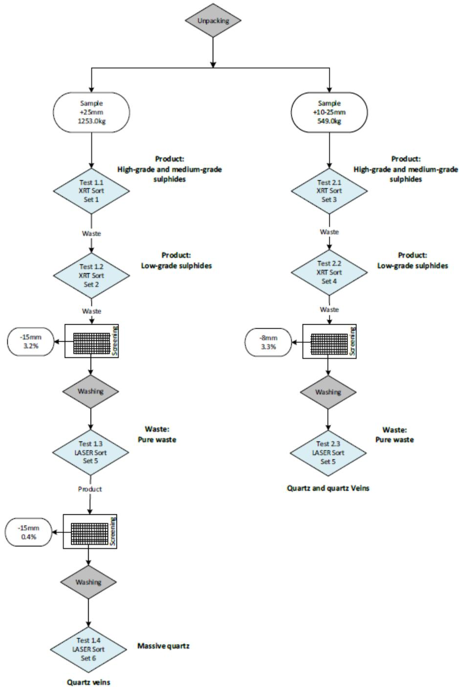
Figure 13-12: Mineral sorting testwork flowsheet
