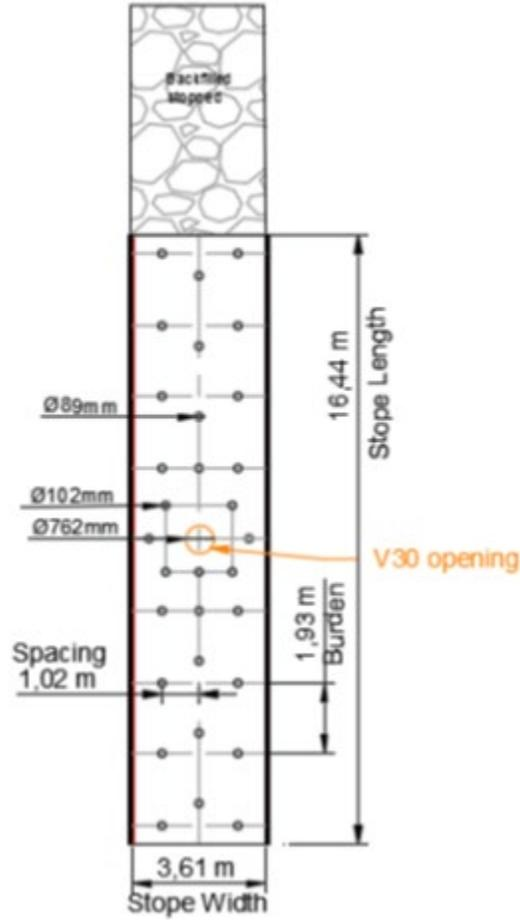
Figure 16-17: Typical drilling configuration for Valley Zone, plan view
