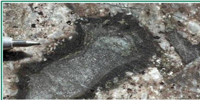
Biotite rim retrograde to skarnified wall rock clast in intrusion breccia
