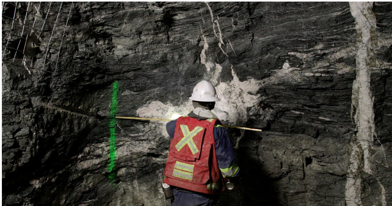
Figure 1: Visible sulfide mineralization in the bottom sill development.
